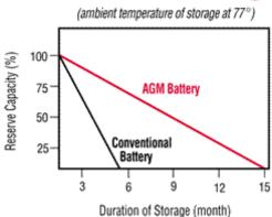
Because of its lead calcium design, the AGM battery will hold its specific gravity more than three times longer than conventional lead antimony types. This means much longer periods between charges when the battery is used in a standby mode, like winter storage.
